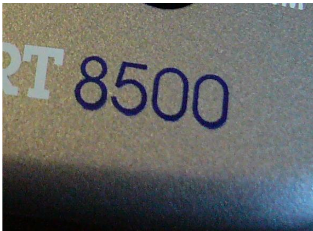
Smudging at the bottom of the “0” – Reject
